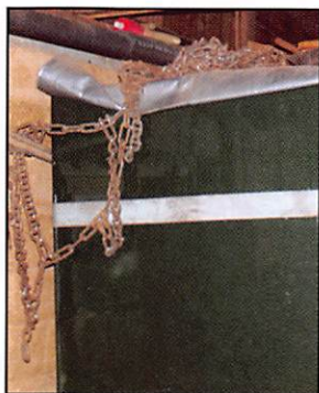
Photo 4 shows how I rigged a large digging or pry bar behind the safe and used my snow chains to extend the length of the chain out to the front of the safe.
