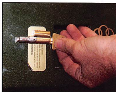
Photo 3 is an American 2000 cylinder on the face of the door showing the location of the cylinder in the safe. The first hole I drilled was a little to the side and above the cylinder connection for a scope hole.
