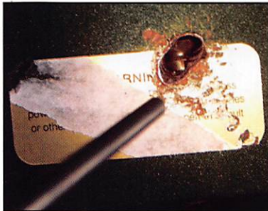
Photos 7 and 8 show the drilled hole, first with the bolt partially spun and next with it dropped out of the locking position.
